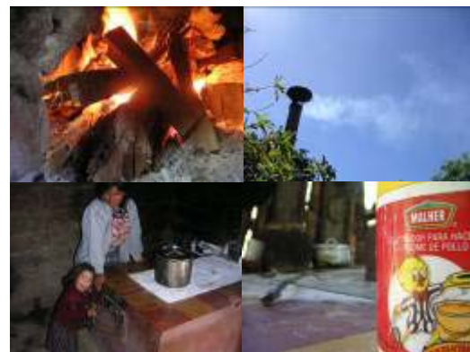
Figure 1: Shown are the plancha (clockwise, beginning at top left): combustion chamber; exhaust flue; work surface; and placement in a household kitchen.
